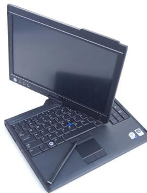
*Figure 3.* Dell Latitude XT2 - a convertible tablet with a multi-touch screen capable of running a full Windows OS and full suite of software. The XT2 has a 12" screen and weighs 3.6 lbs.
